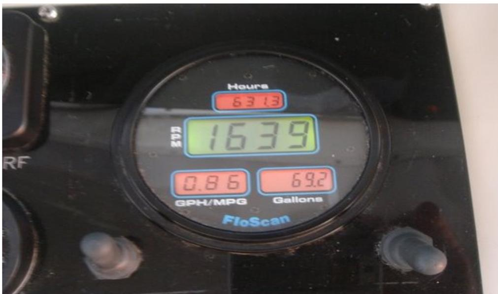
This is the flow scan for the port engine showing .86 GPM at 9.6 knots; the stbd engine floscan was set to show GPH, and at the time of this photo showed 5.1 GPH, which was the same for port at same RPM. Each show cumulative gallons used per engine. MPG is in nautical miles.
